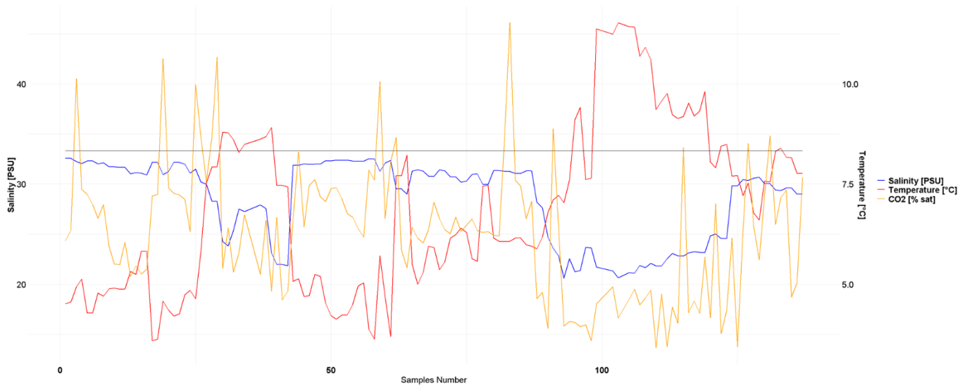
Figure 17. Salinity [PSU] (blue), water temperature [°C] (red) and percentage of saturation of dissolved CO 2 (orange).
