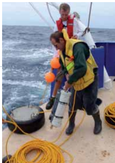
Preparing to deploy a deep water mooring receiver assembly in Australian waters. (Stephane Kirchhoff, OTN Headquarters, Dalhousie University)
